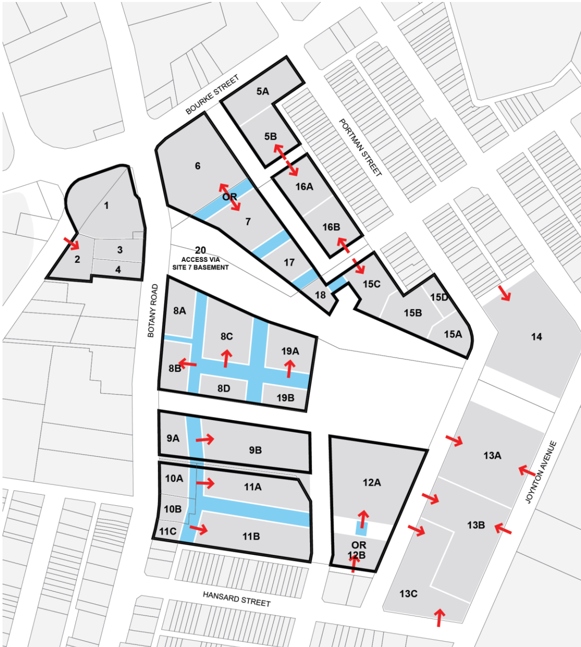
Figure 10.2: Integrated basement car parking
